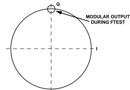
Figure 2. Modulator State During FTEST
